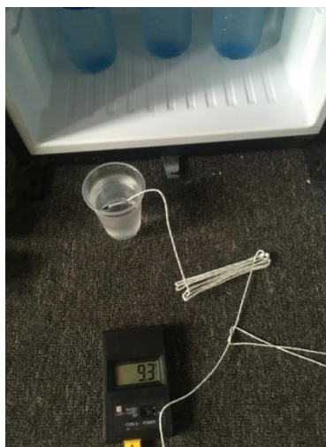
Figure 7. The temperature of cold water obtained using the developed VAR System in this study
