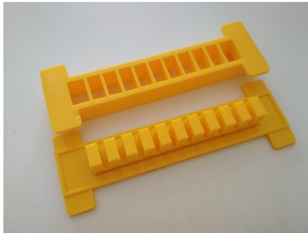
Figure 2: 3D printed molds of the soft actuator
