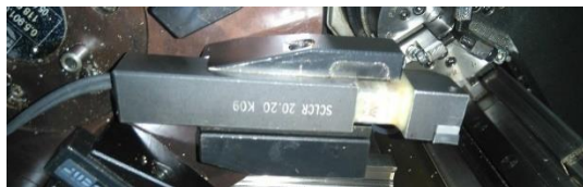
Figure 2: The turning tool with strain gauge[9]
