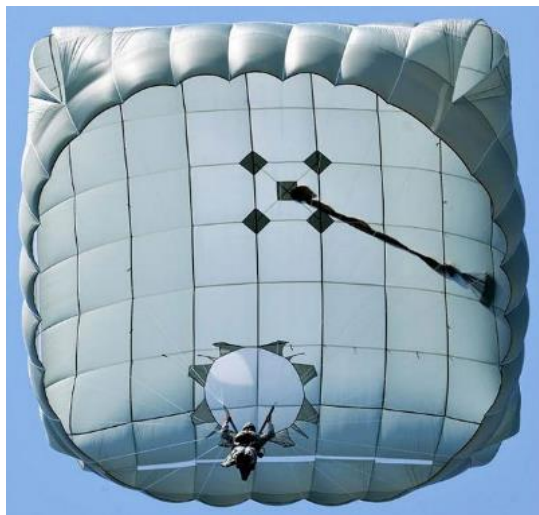
Figure 27. Descending paratrooper under the canopy of T-11 main parachute. On the upper part of canopy surface can be seen the pilot chute and the deployment sleeve [37]
