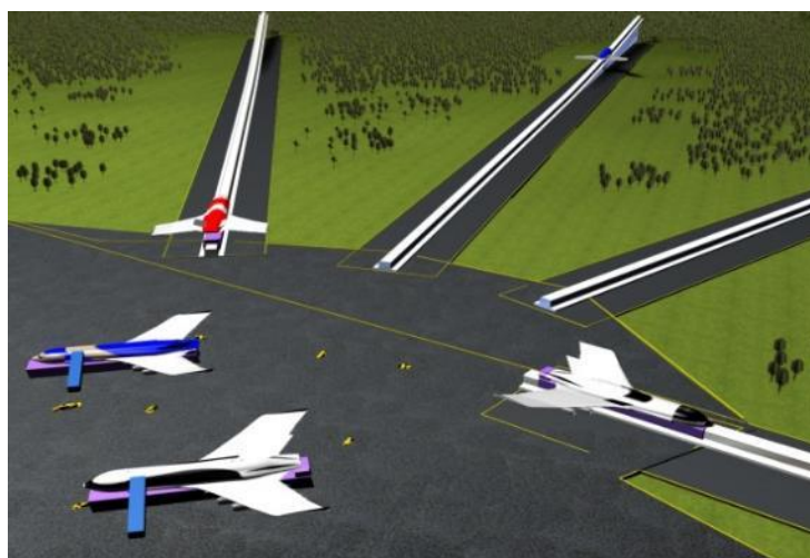
Fig. 10. The use of magnetic levitation technology to to assist the aircraft take-off and landing [22]
