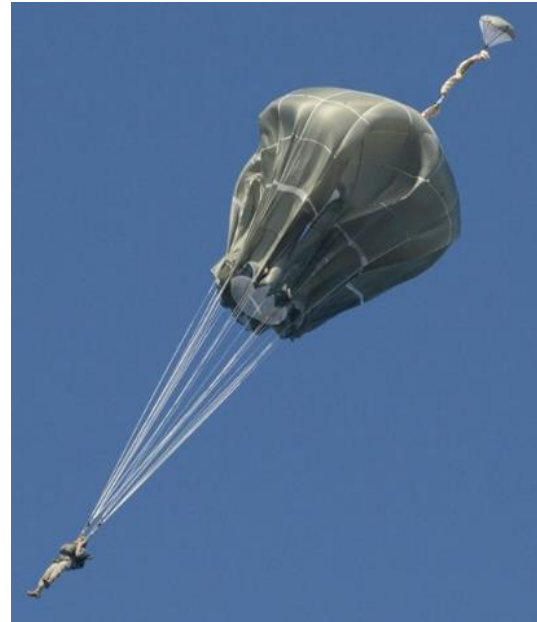
Figure 18. A snapshot about the deployment of T-11 system's main parachute. The pilot chute can be seen on the top of the parachute canopy [25]
