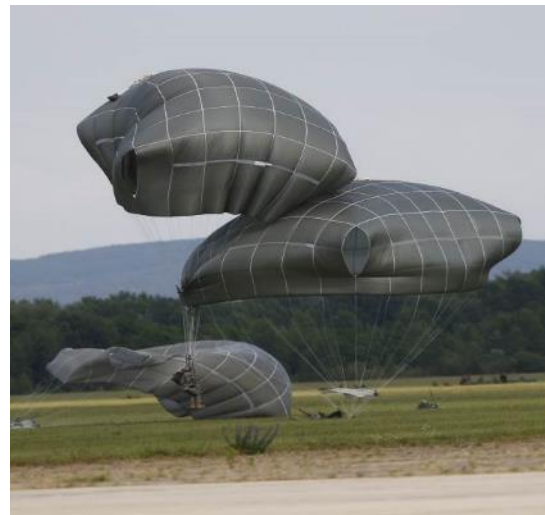
Figure 28. Bad experience: the landing paratrooper slipped through the corner's hole of his comrade's T-11 main canopy during the descent phase. Fortunately the landing ended without injury [38]
