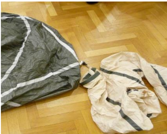
Figure 20. The T-11's pilot chute, connector link and deployment bag of its main canopy [27]
