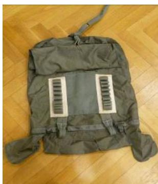
Figure 15. The front and the back side of the T-11's deployment bag and static line [22]
