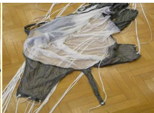
Figure 16. The T-11's special formed slider made from web fabric [23]
