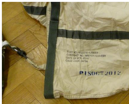
Figure 21. The identification signs on the deployment bag of T-11 canopy [28]
