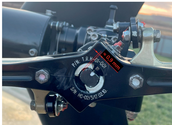
Figure 17. Effect of flapping compensation [13]
