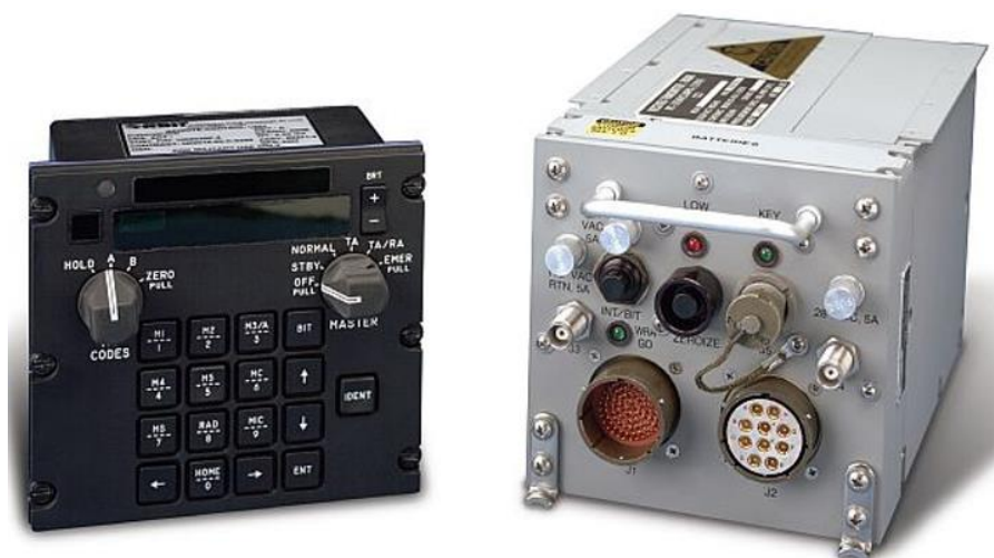
Figure 3. Mark XIIA AN/APX 123/A(V) IFF system 25
