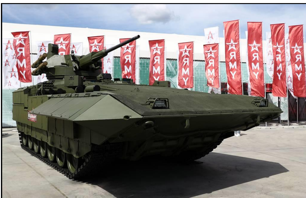
Figure 8: Russian T-15 armoured infantry fighting vehicle on Armata chassis with EPOCHA turret [27]
