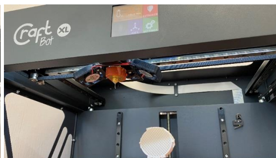
Fig. 4. 3D printing, demonstrating the internal structure of the given object
