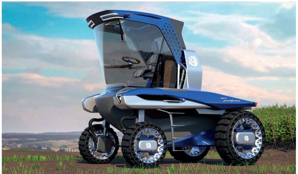
2. kép. New Holland Straddle Tractor Concept hidas traktor formaterve (forrás: https://pininfarina.it/en/work/straddle-tractor-concept/ )
