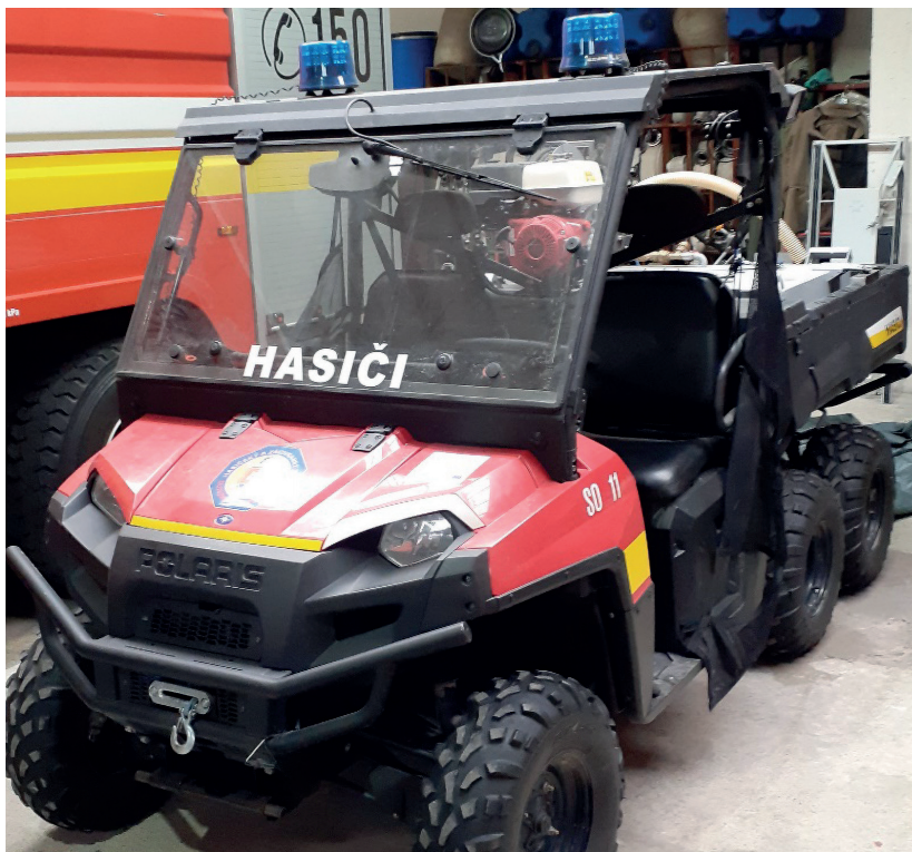
Picture 4: An ultralight fire vehicle on duty in Slovakia
