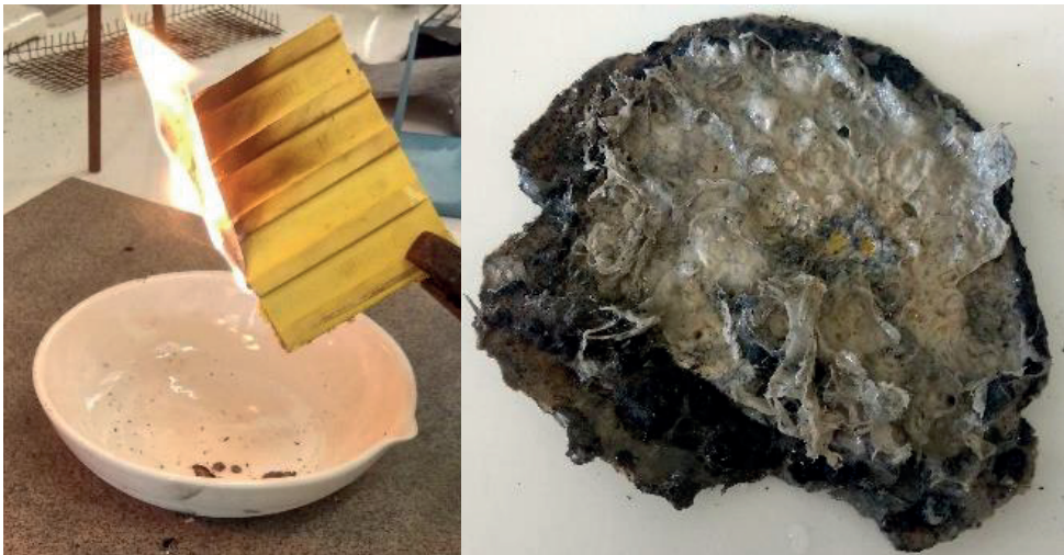
Figure 6: Behaviour of sample during the burning process and burning residual
