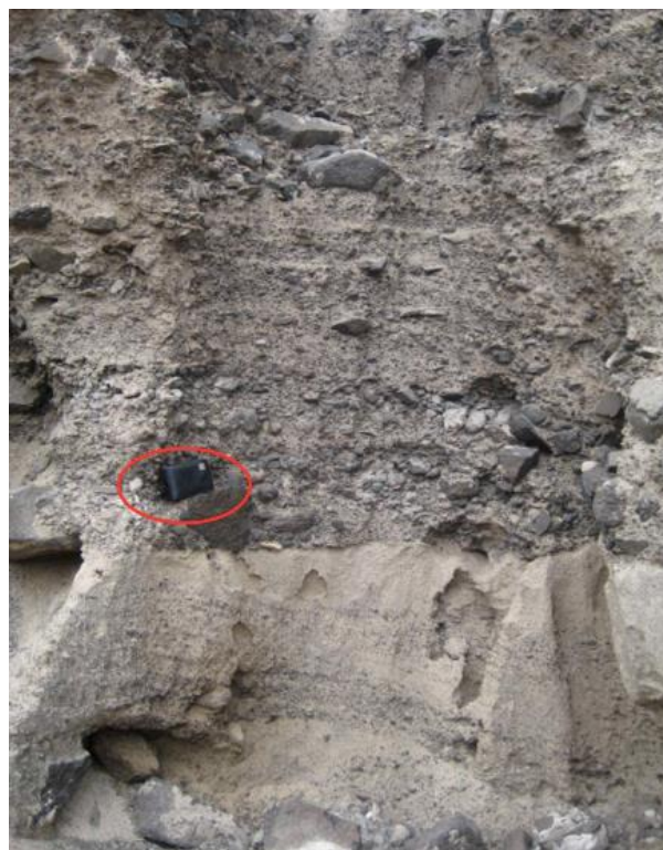
Fig. 5 Typical profile where we see colluvium and lower down wind-blown deposit. The box of the camera surrounded by the circle serves as a scale
