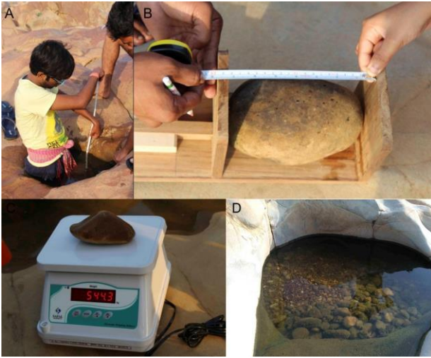
Fig. 6 A. Pothole where depth is greater when compared to aperture diameter. B. Dimensions measured with the help of a specially devised instrument. C. Weight measurement of grinding stones D. Pothole almost full of stones quoted with mosses.
