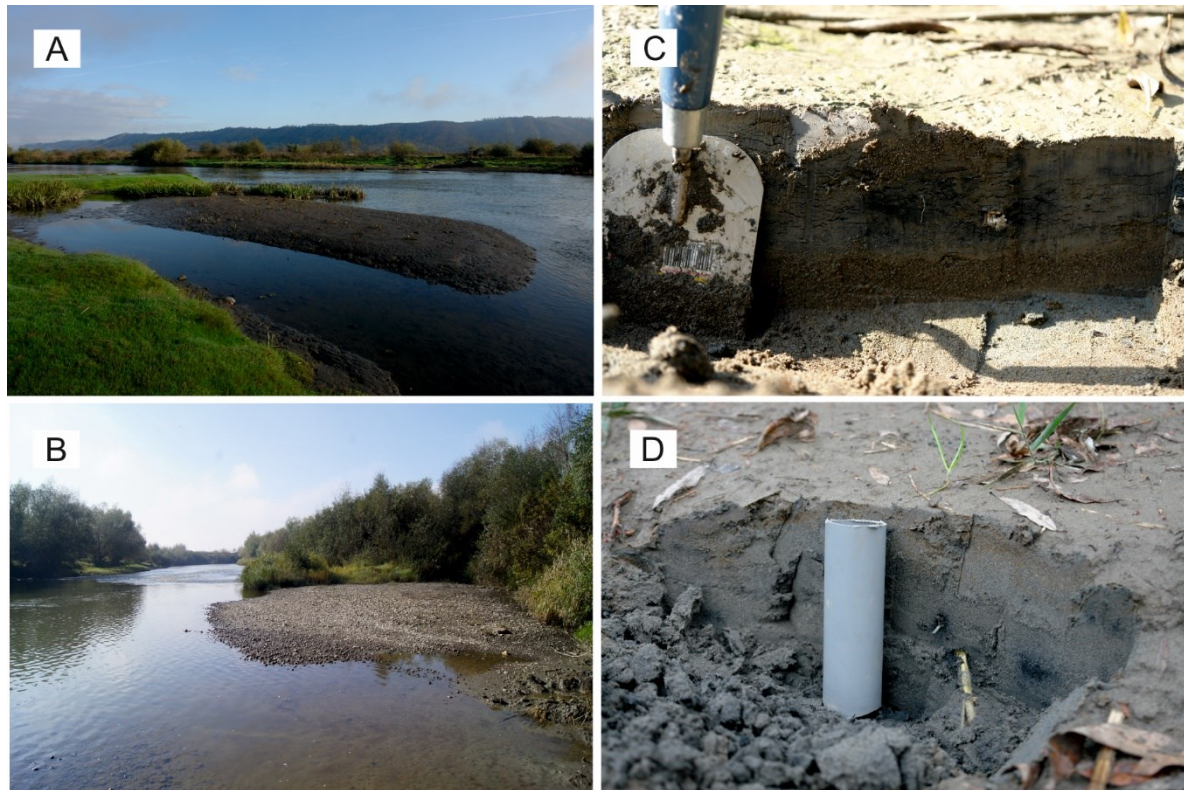
Fig. 2 Typical sample collection sites include point bars (A) and side bars (B). Sampling was performed from the uppermost, thus freshly deposited sediments by spatula (C) or plastic tube (D) for undisturbed samples.
