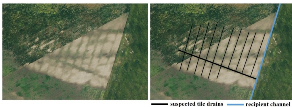
Fig. 4 Appearance of tile drain lines near Kunszentmárton, Hungary. The drawn lines on the bare soil continue on the surface with vegetation too, where the lines still could be observed due to differences in vegetation growth or species composition (source: Institute of Geodesy, Cartography and Remote Sensing of Hungary)
