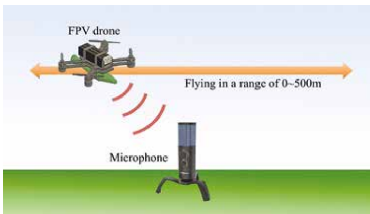
Figure 1: Measurement setup for the audible recording of an FPV drone (Edited by the authors)
