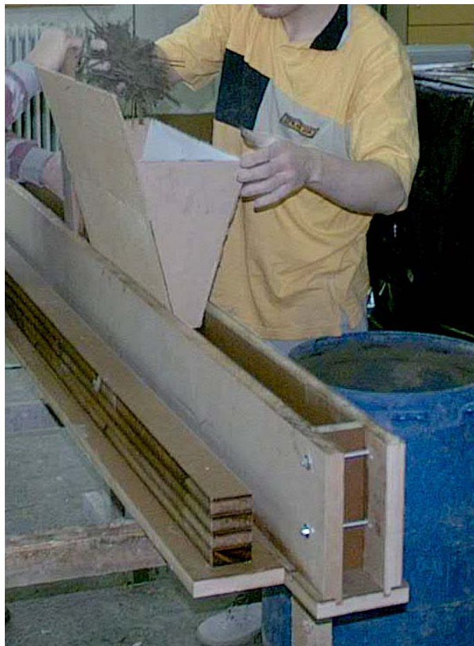
Figure 4. Aligning the strands in LSL type composites
