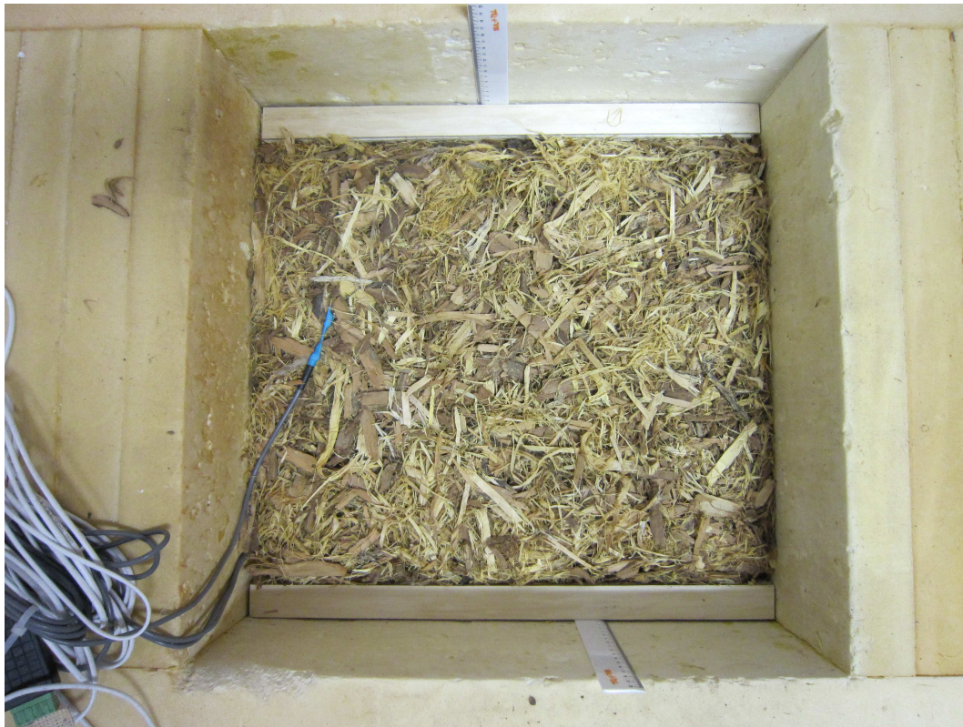
Figure 1. Chipped bark of black locust is placed in the measurement box for testing.
