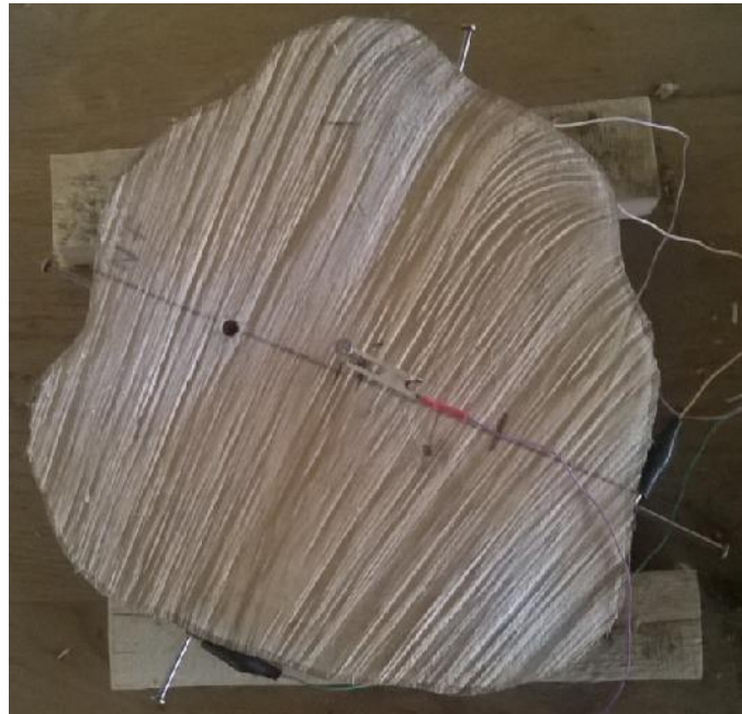
Figure 2. 8 mm diameter bore, drilled into slice of hornbeam for experimental measurements
