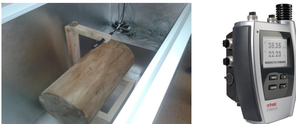
Figure 3. General view of the freezer containing a log (left) and of the Data Logger (right)
