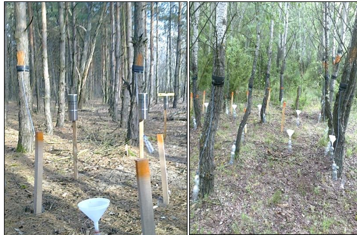
Figure 2. Trunk collar system with Hellmann rain gauge unit
