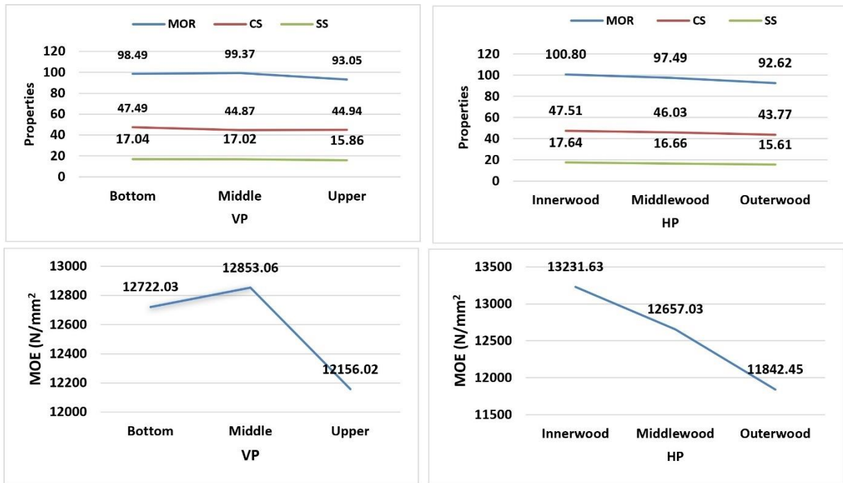
Figure 5. Showing the mechanical properties ( N/mm^2 ) within VP and HP for A. leiocarpus . (VP): vertical positions; (HP): horizontal positions; (MOR): modulus of rupture; (MOE): modulus of elasticity; (CS): compressive strength parallel to the grain; (SS): shear strength parallel to the grain
