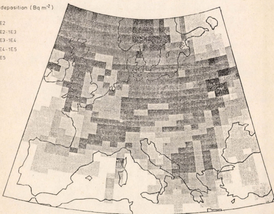
Fig. 3: Accumulated estimated deposition of \text{Cs}^{137} between 26. 4.86 and 15.5.86 from MESOS – II simulation
