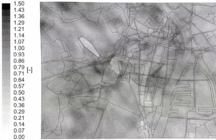
Fig. 6. Distribution of the velocity magnitudes scaled by reference values (inlet profiles) in the examination area, at 30 meters above the ground.
