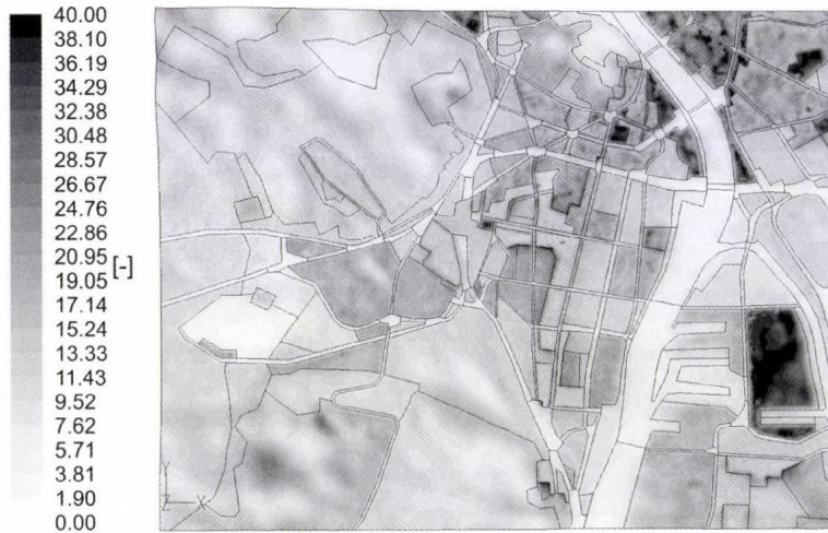
Fig. 7. Distribution of the turbulent intensity scaled by reference values (inlet profiles) in the examination area, at 10 meters above the ground.
