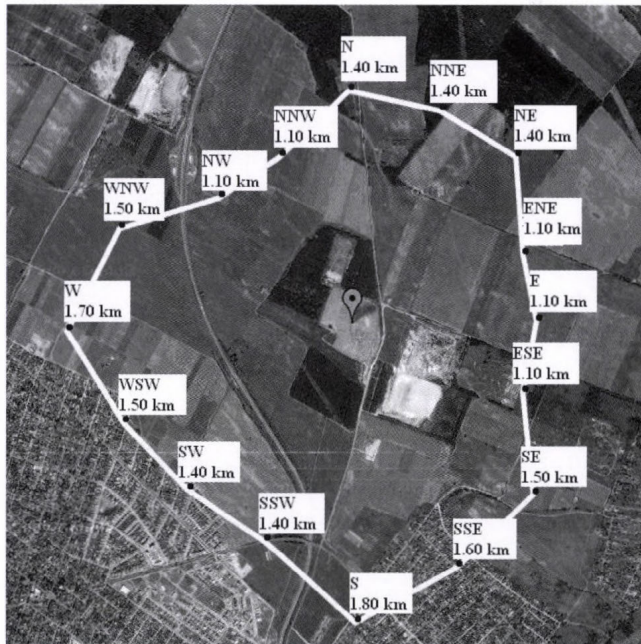
Fig. 2. Odor setback distances along the 16 wind directions around a municipal solid waste landfill in Dunakeszi, Hungary.
