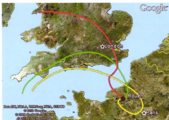
Fig. 8. PyTRES trajectories started from Rouen at 07 (red), 13 (yellow), and 22:30 (green) UTC, January 21, 2013. Meteorological conditions allowed the plume to spread towards Paris only within a few-hour long time period.
