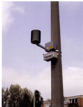
Fig. 3. One of the stations of the monitoring network on a lamp post (temperature and relative humidity sensors are inside of the radiation shield cylinder).
