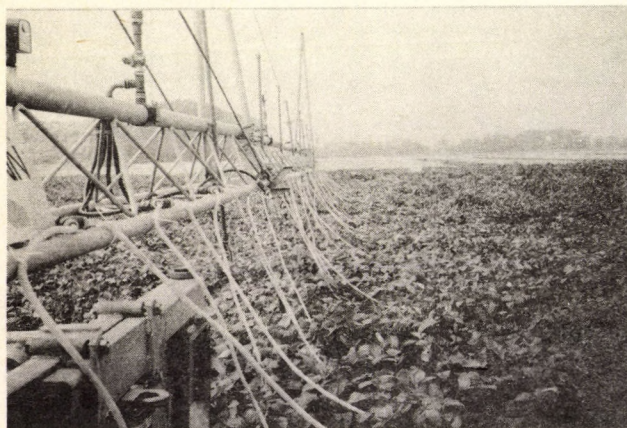
Fig. 2.: The flexible tubes for surface irrigation
