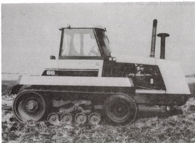
Fig. 1. Caterpillar Challenger-65 with rubber-belt track-drive.
