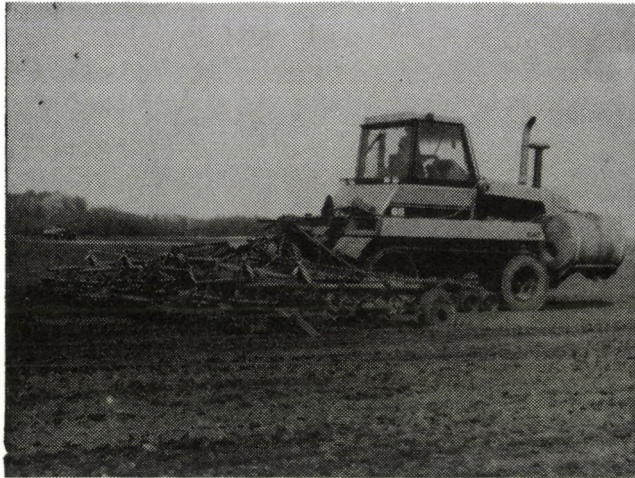
Fig. 4. Challenger-65 tractor with RAU-Unimat 8,4 seedbed preparator
