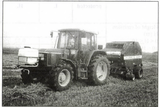
Fig. 1 Dispensing of additive and baling
