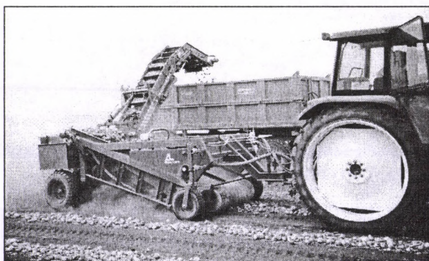
Fig. 4 ASA-LIFT onion pick-up
