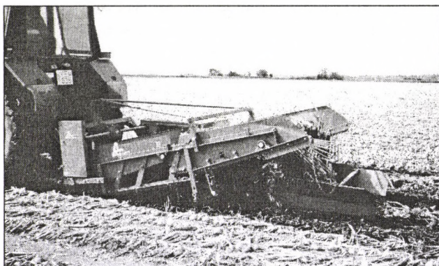
Fig. 3 ASA-LIFT onion lifter
