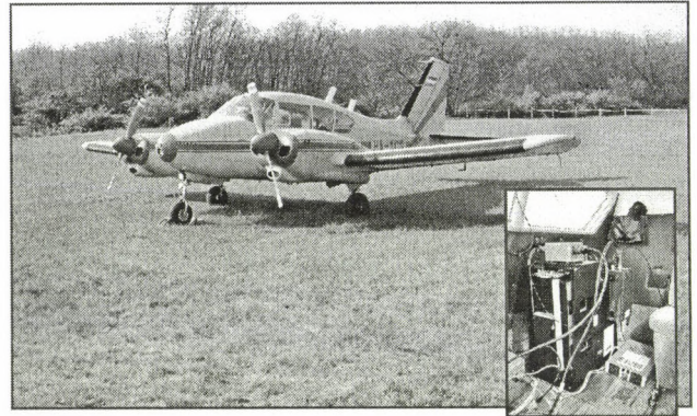
Figure 3 PIPER AZTEC airplane and Hyperspectral sensor with OxTS RT3003 GPS/INS unit
