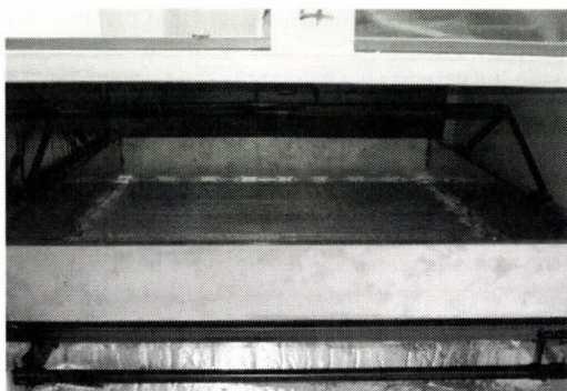
Figure 3. Shelf and heater of the experimental dryer
