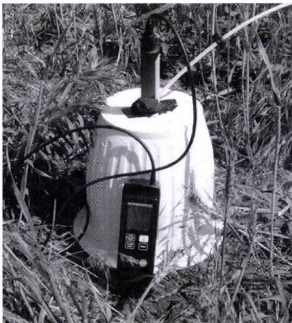
Figure.2 TESTO 535 CO 2 tester and “C02” portable chamber
