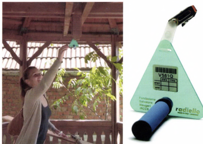
Figure 1. Radiello passive monitor probe and its allocation
