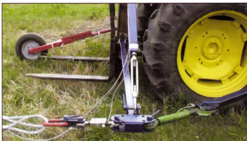
Figure 3. Purpose-designed drawbar mechanism with a converted forklift.
