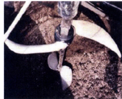
Figure 3. Combination of vertical bladed and propeller stirring fans [5].
