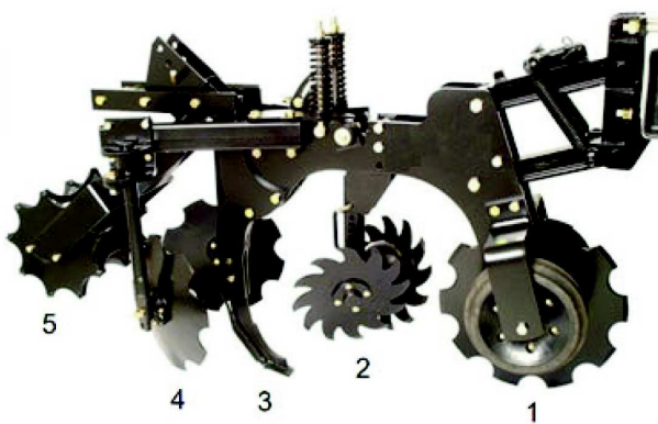
Figure 1. Basic components of a typical strip-till unit include: (1) opening coulter; (2) residue managers; (3) mole knife/NH 3 injector; (4) covering disks; and (5) seedbed conditioner. (Photo courtesy of Yetter Manufacturing, Hagenstaller, 2103)
