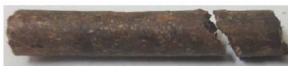
Figure 8. Longer pellets beginning to break from the end
