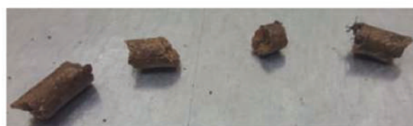
Figure 9. 50-25-25% Acorn-Pine-Sawdust mixture ratio 40 \text{ mm} < \text{PL} \leq 45 \text{ mm} Length Class Pellet
