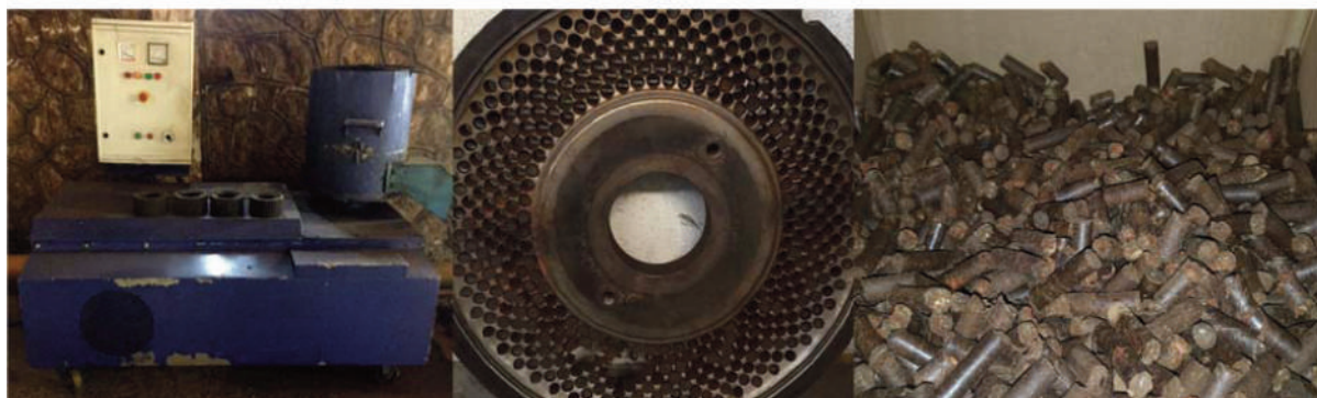
Figure 3. Pelletizing machine with 8 mm disc and pellets
