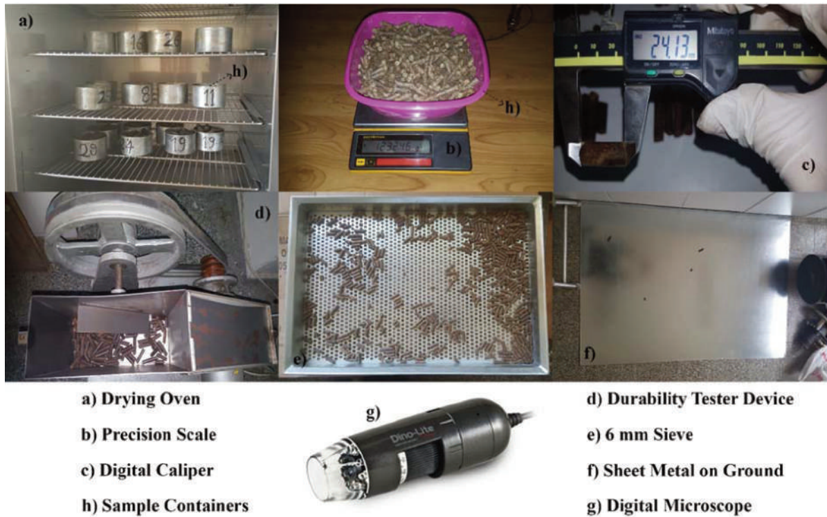
Figure 4. Devices and Equipment
