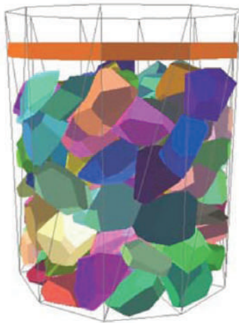
Figure 7. Initial state of the polyhedral pack before the pressing process
