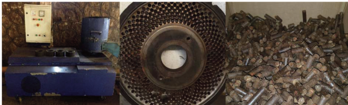
Figure 3. Pelletizing machine with 8 mm disc and pellets
