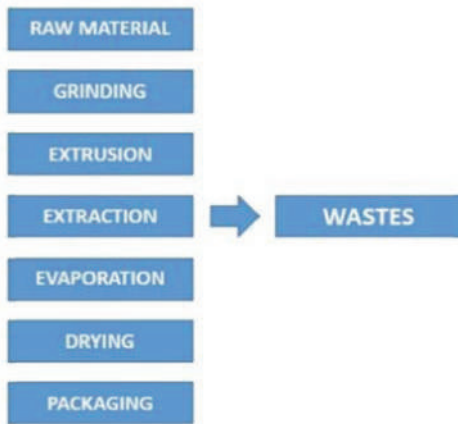
Figure 1. Valonia production process
