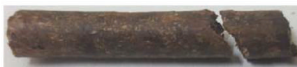
Figure 8. Longer pellets beginning to break from the end
