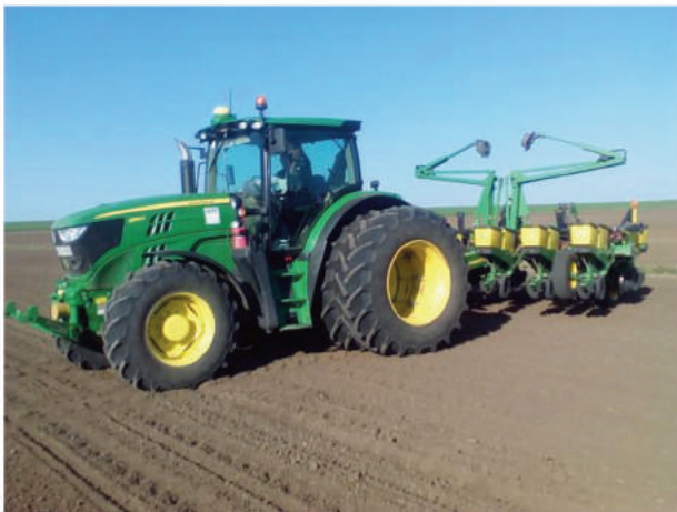
Figure 2. An John Deere 6150R with the StarFire 3000 Receiver (The photo has been made by the authors)
