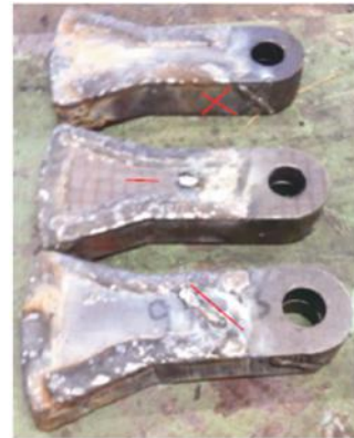
Figure 10. Hard metal welded hammers
