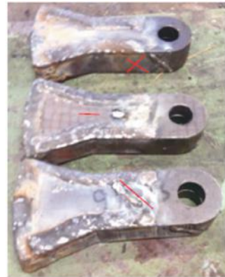
Figure 10. Hard metal welded hammers
