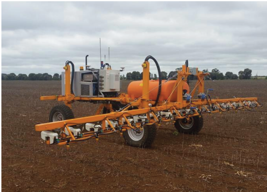
Figure 7. 4WD SwarmFarm robots carrying WeedSeeker technology cover the paddock spraying only living weeds Source: (Bloomer, 2017)
