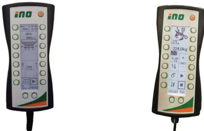
Figure 3. Innovations from INO's Electronic Development Laboratory - INO SmartAssist for FERTI-2 Fertilizer Spreader and for VVP 115 Vibrational Subsoiler with deep fertilizer device (Source: INO)
