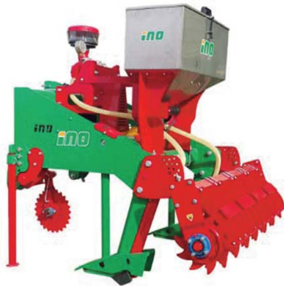
Figure 2. VVP 115 vibrational subsoiler with deep fertilizer device (Source: INO)
