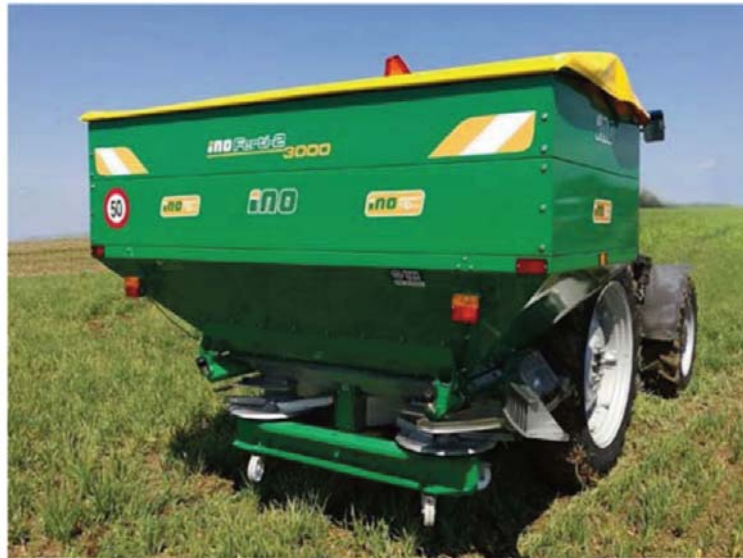
Figure 1. Double-disc mounted fertiliser spreader FERTI-2 (Source: INO)
