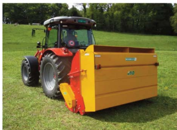
Figure 5. Flail mower INO Smart Hopper (Source: INO)
