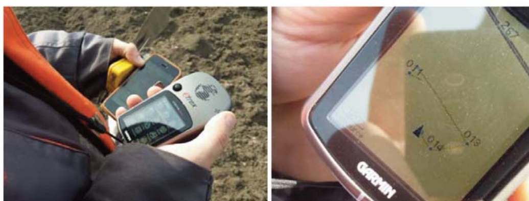
Figure 6. Exact location of the measuring point using the GPS unit
