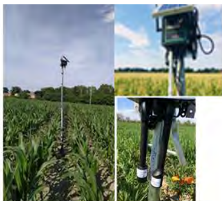
Installed sensors in a research crop field, measured parameters : air temperature, humidity, pressure, CO 2 and ammonia
