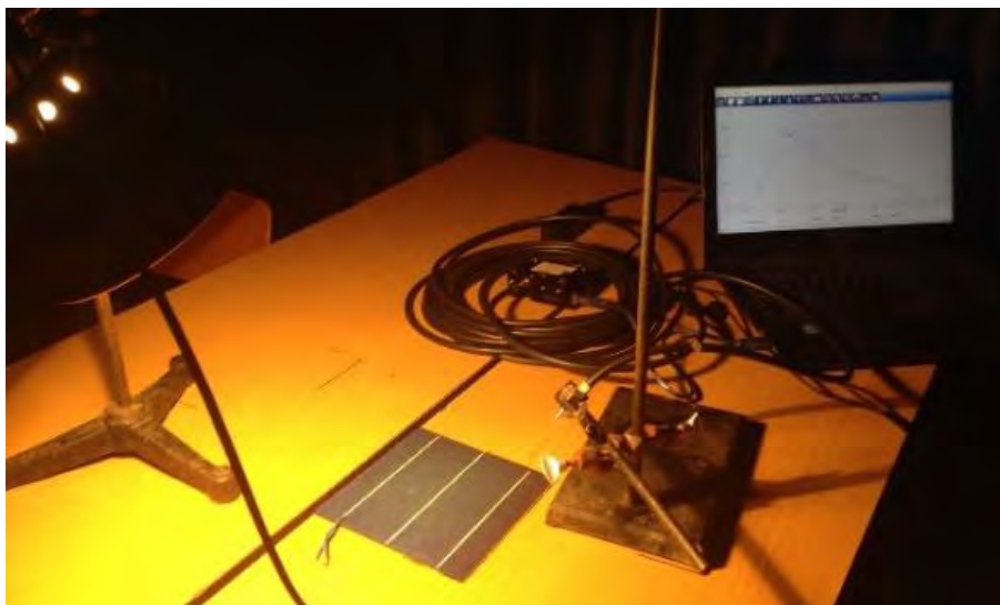
Fig. 8. Experimental layout for measuring the reflected spectrum
