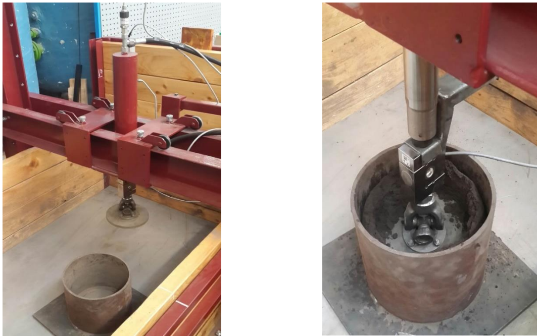
Figure 7. Bevameter test at the university laboratory testing the loam sand soil at different moisture contents
