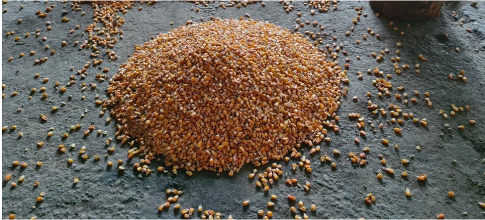
Figure 1. Angle of repose test can be done easily and rapidly anywhere
