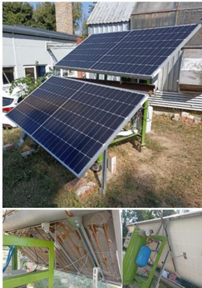
Figure 1. Experimental Setup, Conventional PV and modified PV panels
